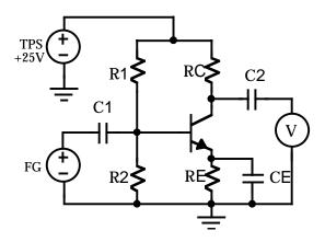
You will have designed and built this circuit earlier, having chosen the resistor values to provide a stable operating point and relatively large voltage gain. Capacitors  $C_1$  and  $C_2$  will be about 10  $\mu$ F, and  $C_F$  will be around 100  $\mu$ F to maximize the midband gain.
